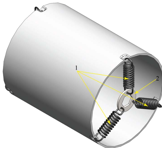
Fig. 4 Stainless steel drum for smoothing the ski running surface (1 - spring hanger, 2 - mounting washer)
