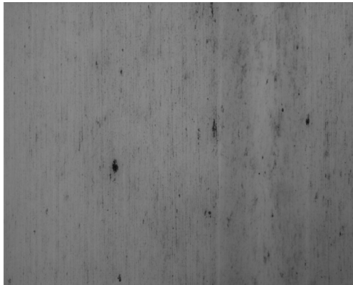
Figure 12: Waxed with Swix ® CH8 after 3.8 km (Case4)
