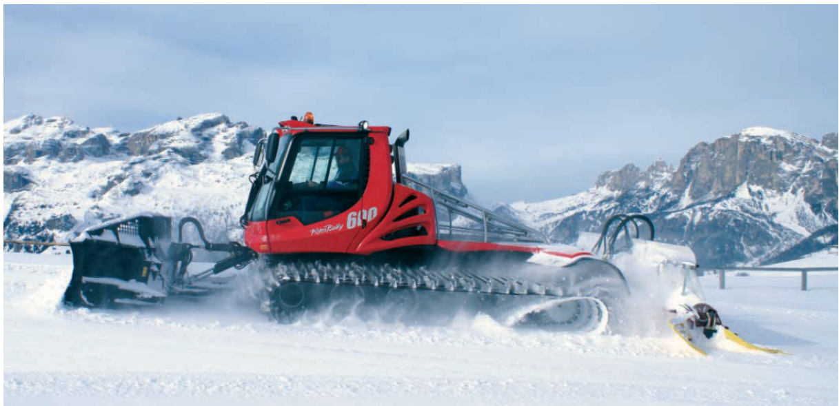
Figure 4: Grooming machine with front blade and lowered snow tiller (brochure Pistenbully 600 9 ).
