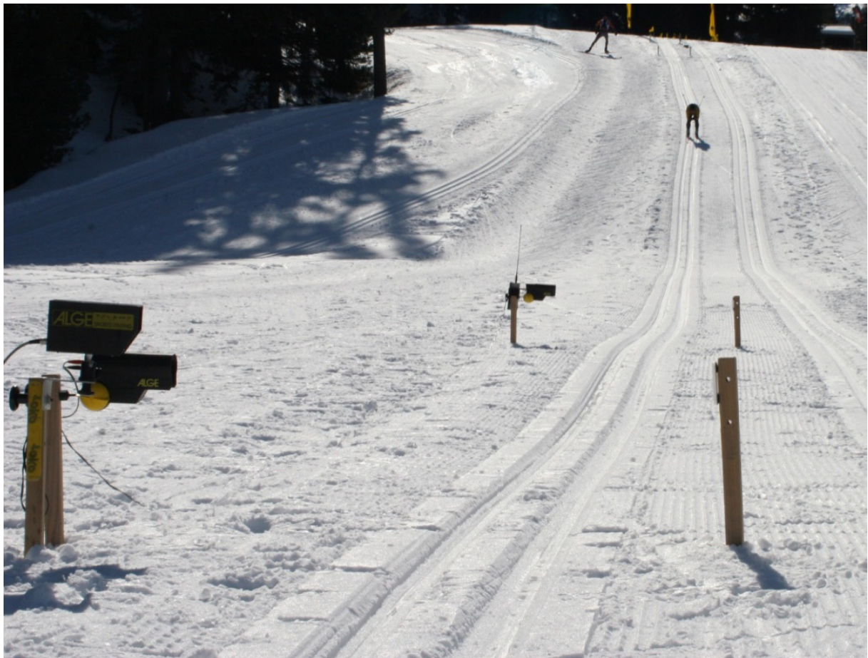
Figure 17: Typical test setup for Nordic skis. The additional light barriers at the start and finish of the track are used for the determination of the start and final velocity.
